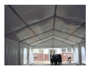
The A-frame is extendable in length and available in 6m, 9m, 12m, and 15m standard widths.
